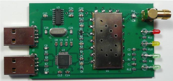
Figure 4 – SHARI PCB with all Components Installed
