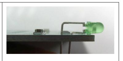
While holding the LEDs so they do not fall out, turn the board over on a flat surface. Align the LEDs so they are perpendicular to the end of the board. Ensure that they protrude an equal length from the board and that the annular rings at the base of the LEDs do not protrude beyond the edge of the board.
