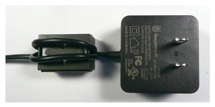
Split Core Ferrite Installed on Raspberry Pi Power Supply Cable (three turns)
