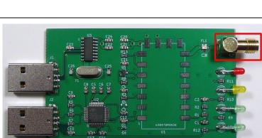
Next, you will solder the SA818 radio module to the PC board in the U1 position. You will solder 18 castellated hole on the module edges to the pads on the PCB. If you have never soldered castellated holes before, please go to
