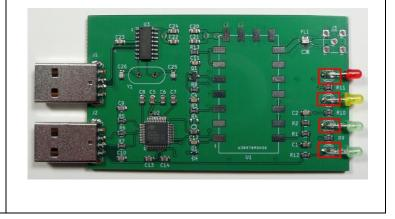
Insert the crystal, Y1, into the PC board from the top as shown in the photo. Solder the two pins on the bottom side of the board. Trim excess lead length.
