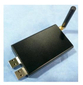
Figure 2 – SHARI has Two Type A Male USB Connectors for the Allstar Interface and Radio Programming
