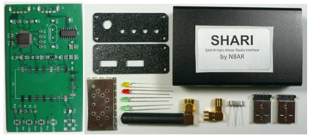
Figure 5 – SHARI Kit Components (included ferrite filter not shown)
