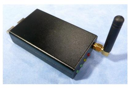
Figure3 – Four LEDs indicate the Status of Power, Allstar USB Interface, Radio COS and Radio PTT
